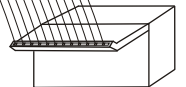
AQUA SPRAY Part # G A 1 2 _____ SINGLE ROW SPRAY AT 60 DEGREE ANGLE: Sprays out To 12' and 1.5 to 4' high. RATE: 3 - 7 GPM also available in Vinyl pool design nozzle
